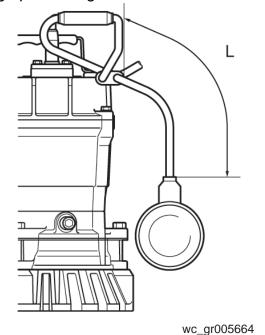
2.4.1 Set the length of the float lead wire to the dimension indicated below. Failure to set the correct lead wire length will lead to improper operation of the pump.
