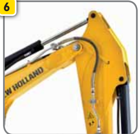
Reinforced boom/arm connection
