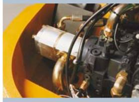
Separate hydraulic pumps provide fast cycle times.
