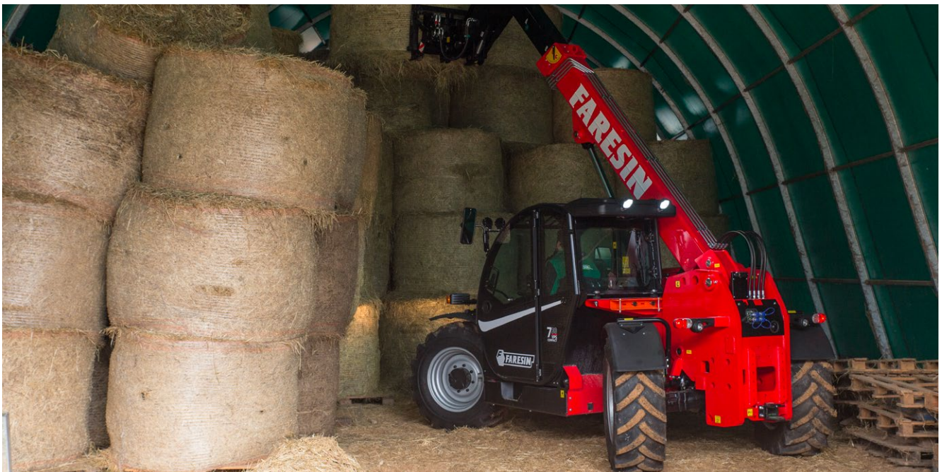
Crab steering for side approaches and delicate manoeuvres
